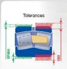
The EF800 specification sets out reduced bore tolerances for the cylindrical bores, for the tapered bores, for the outer diameters and for the radial clearance, compared to the tolerance ranges of the normal series. See table below.
