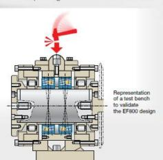
The many tests carried out on the NTN-SNR test benches have demonstrated the excellent behaviour of our bearings when subjected to intense vibratory conditions.
